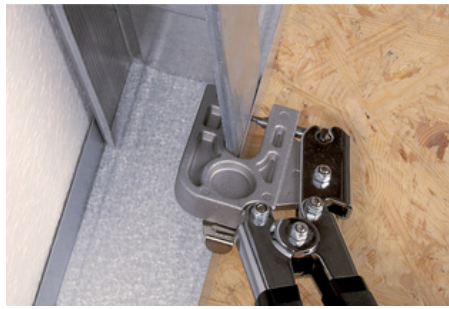
afb. 07.1.1 - 10 Professionele klinktang -> professional crimp pliers
